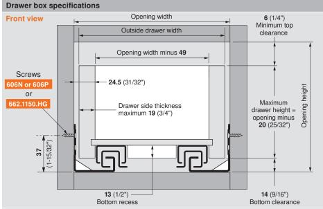
**NOTE:** Drawer side material thickness may vary. Accurate measurement of drawer side material thickness should be used when calculating outside drawer width using the table below. Inside drawer width **must** equal opening width minus **49** (1-15/16") for TANDEM to align and function optimally.
