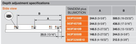
Mount each runner using at least two of the elongated holes. Install the drawer to check the position of the drawer front.
